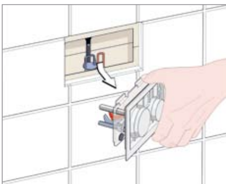
For servicing, the complete unit with lever mechanism, cover, splash guard and mounting plate can be removed. All settings are retained.
