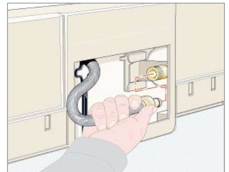
After the shell construction stage: The reinforced pipe is attached to the plug connection on the filling valve with no need for tools.
